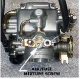
If it is a screw head, skip to step #11c. If you see a brass plug with a small hole in the center, proceed as follows:
