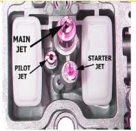
9. Thoroughly clean the inside of the float bowl prior to reinstalling it.
