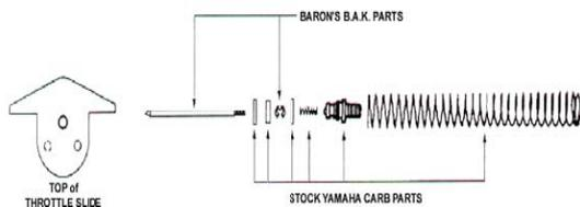
5. Reinstall the vacuum slide along with the diaphragm spring.
