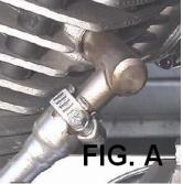
Next, remove air injection pump along with all associated rubber lines and brackets - for Road Star applications refer to (Fig. B & C).
