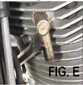
*NOTE:* The air fittings are very tight in the cylinder head. We have found that when driving out the air fittings, the 90-degree joint may start to tear apart. If this happens, simply insert your removal tool into the hole in the
