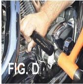
Insert the tool into elbow area of the air fitting and FIRMLY drive the fitting from cylinder head with a hammer (Fig. E).
