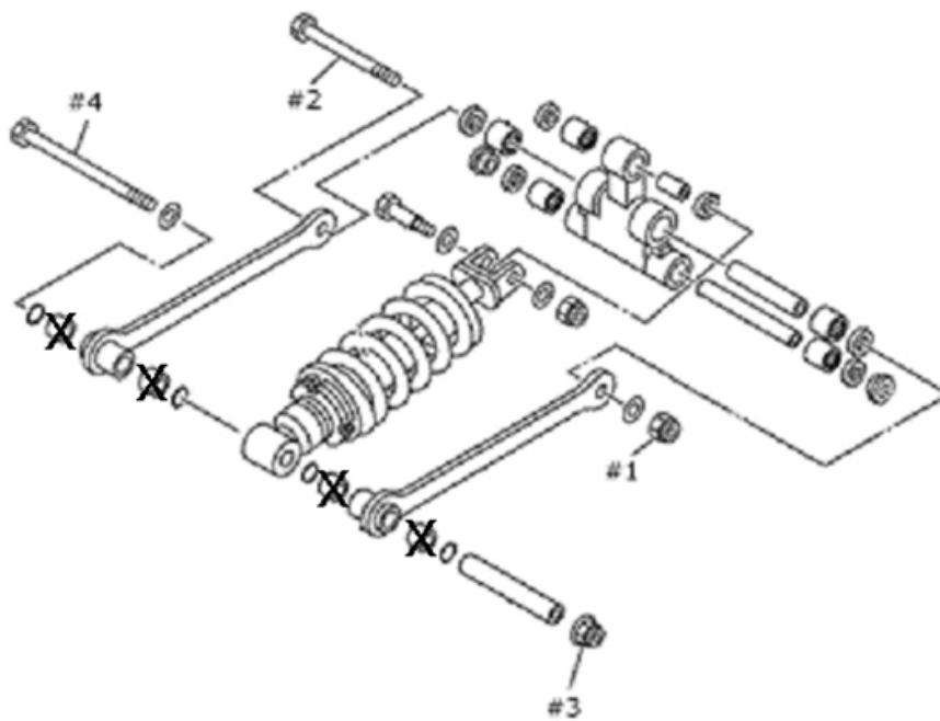
**NOTE:** We recommend that you set the shock spring preload to a higher setting, especially if the motorcycle will be used for carrying a passenger or heavy loads.
