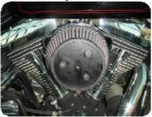
5. Lastly, place the chrome screen into the xXx cover and install over the air filter using the supplied polished flat head bolt and Loctite. Tighten the bolt, clean off the cover and around the air cleaner assembly. Installation is complete. Be sure to clean and re-oil yair filter on a regular basis. Also, be sure to re-torque bolts after riding to ensure air cleaner assembly remains secure.
