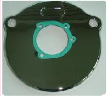
2. Mount the large chrome backing plate to the cylinder heads via the supplied chrome spacers and breather bolts. Spacers have a lip that helps them seat flush in the backing plate. Be sure to use Loctite when securing the bolts. For Evo engines use the larger 1/2-13 breather bolts. For twin cam engines, use the 3/8-16 breather
