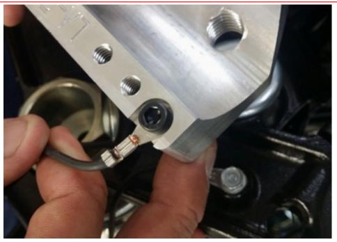
Next secure the ground wire with supplied 10-32" bolt. You must do this before installing the top clamp. *Note:* You'll want to put the top clamp on next, snug it up with a couple bolts, and test putting the nacelle cover back on to make sure the ground wire is in a good location that will clear and not be pinched.
