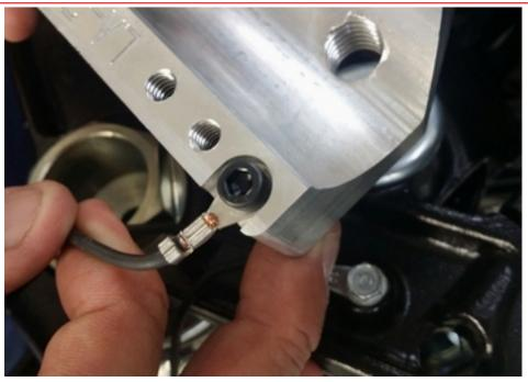
Next secure the ground wire with supplied 10-32" bolt. You must do this before installing the top clamp. *Note:* You'll want to put the top clamp on next, snug it up with a couple bolts, and test putting the nacelle cover back on to make sure the ground wire is in a good location that will clear and not be pinched.
