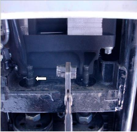
3. Raise the rear wheel about three inches. This will pull the shocks back. This will create enough room to install the split collars in Step 4.
